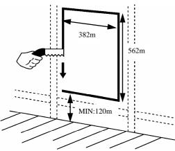
3. Carefully place the sheet metal frame into the hole and make sure that it is flat and square. Secure the sheet metal frame with screws or by bending the metal tabs over the gyprock sheeting.
