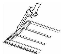
4. Ensure the grille is in the correct orientation (filter opening should be at the bottom). Carefully push the grille through the hole and ensure that it is flat and square. Support the frame in the required position while the adhesive sets.
