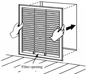
5. To clean the filter, simply slide the whole filter out of the grille frame and wash with warm soapy water.
