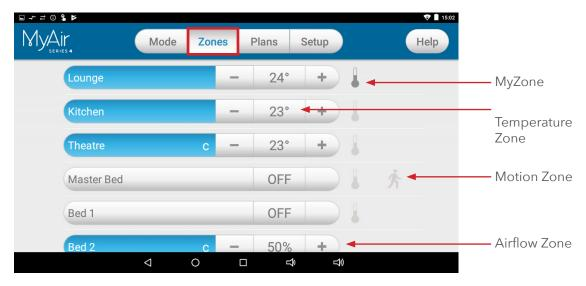
Pressing a zone name toggles that zone between ON and OFF. Zones are ON when they are the blue colour.
